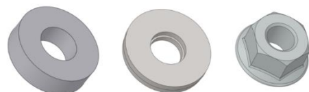
Spacer (left), Nut washer (middle), Nut M8 (right)
